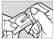
**2** To open the Test Strip packet, carefully PEEL the foil until the Test Strip is completely exposed (as shown).
